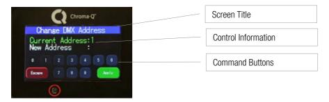
The screen shows the current DMX start address and the new DMX start address. In the screen, the numeric command buttons can be tapped to set the new DMX start address.
