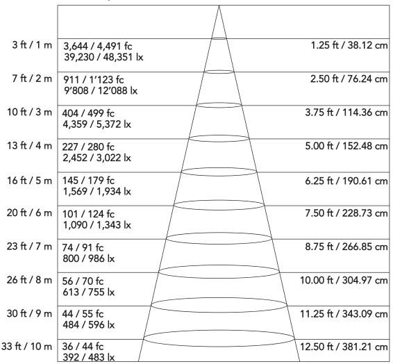
Height Eavg / Emax Angle: 26° Diameter
