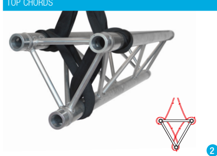
TRIANGULAR TRUSS | APEX DOWN 1 SLING, BASKET ON BOTTOM CHORD AND WRAPS ON TOP CHORDS
