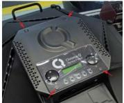
3. Carefully lift the back cover from the unit. The adjusting knobs will slide off with the cover. Remove the 5-pin overlay connector from the PCB board before completely removing the cover. Do not bend the pins. Set back cover aside.
